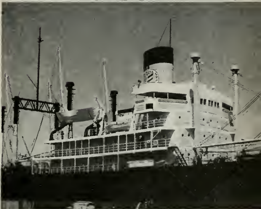
At top: Washington Mail, one of six new 16-knot cargo liners of the 12,800 dw ton class among the fleet of fast ships operated by American Mail Line Ltd. in Oriental service out of West Coast ports. Each ship has limited passenger accommodations. Five are fitted for refrigerated cargo.
